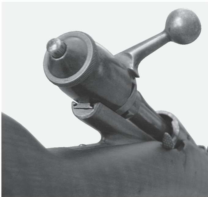
Detail of the bolt rail of a Model 1870/87/15 Carabinieri carbine showing how the modified striker shoe fits neatly in the machined bolt extension rail in a similar way to the "Versione MB". (Roberto Gobetti)
