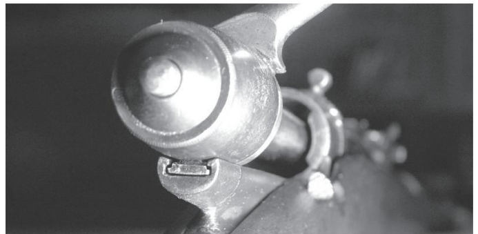
Detail of the "Versione MB" bolt showing how the modified striker shoe fits neatly in the extended bolt support rail. (Jim Dawson)
